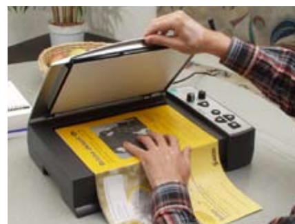
The book edge allows the entire page to lie flat on the scanner.
